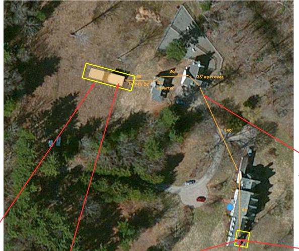
**AC Inverter** Output circuit Underground to Main house.
