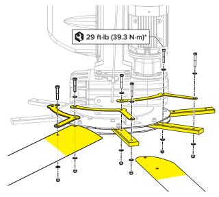
\*If the hardware is stainless steel, ensure bolts are torqued to 10 ft·lb (13.6 N·m).
