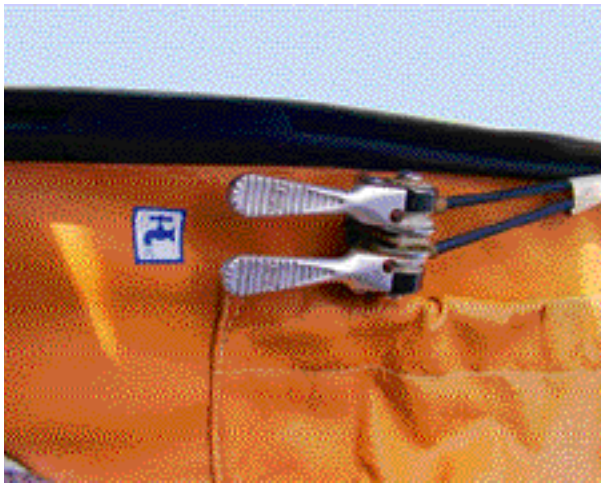
Figure 5-20. Water ballast drain valve handles.
