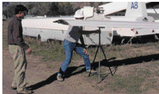
Figure 6-1. Wing stand used during glider assembly.
