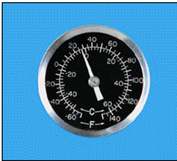
Figure 4-28. A typical outside air temperature (OAT) gauge.
