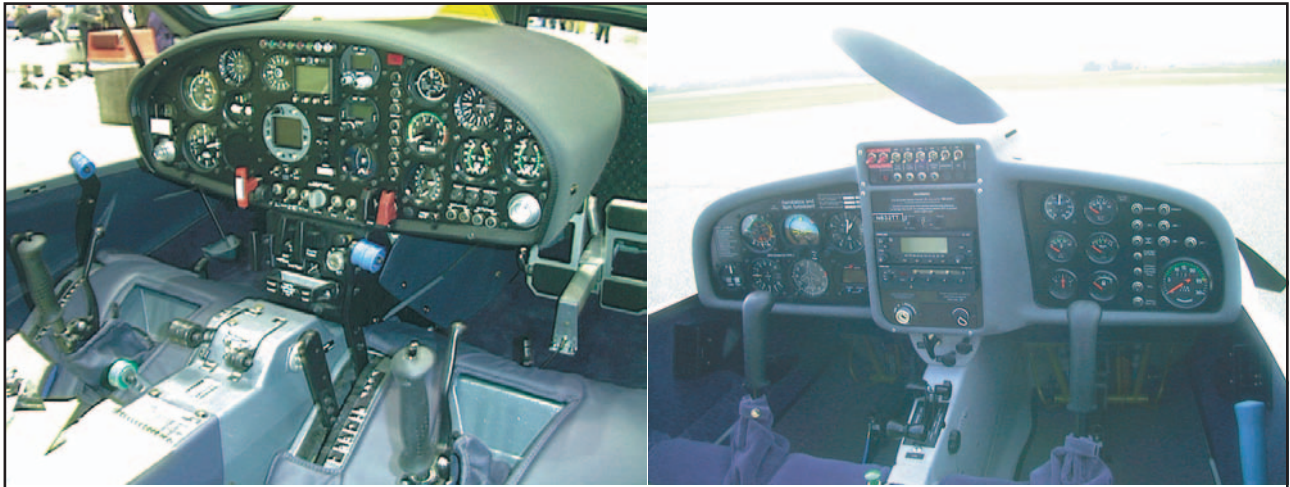
Complexity of the self-launching glider requires a complex instrument panel and a lengthy pre-takeoff checklist.
